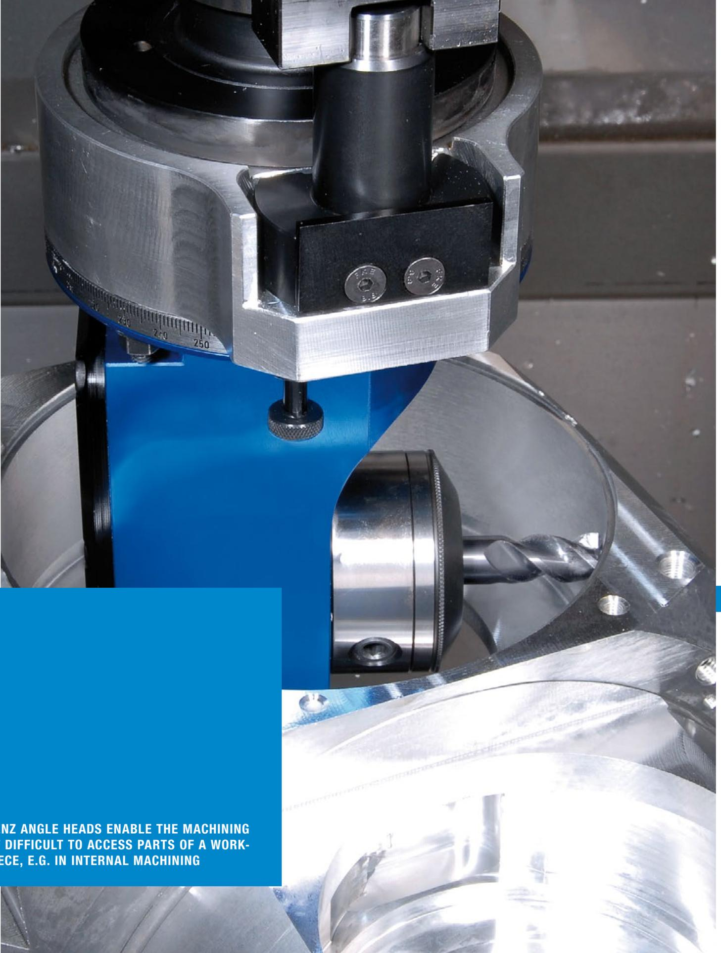
**BENZ ANGLE HEADS ENABLE THE MACHINING OF DIFFICULT TO ACCESS PARTS OF A WORK-PIECE, E.G. IN INTERNAL MACHINING**
